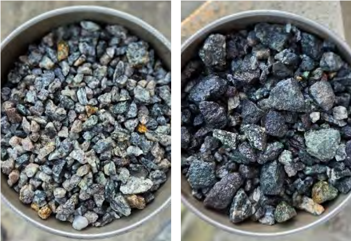
Figure 2: Waste on the left separated from ore grade material on the right.
